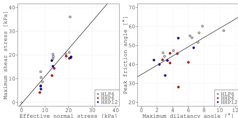
$$\tau_{max} = -0.56 + \sigma' \tan 49.2^\circ \quad \phi'_{max} = 37.7^\circ + 2.44\psi_{max}$$
